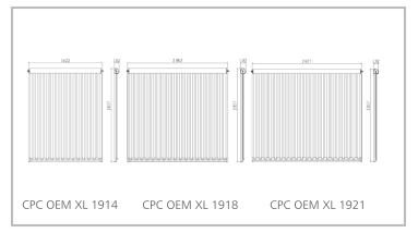
Available in two different tube lengths: 1.50 m and 1.92 m
